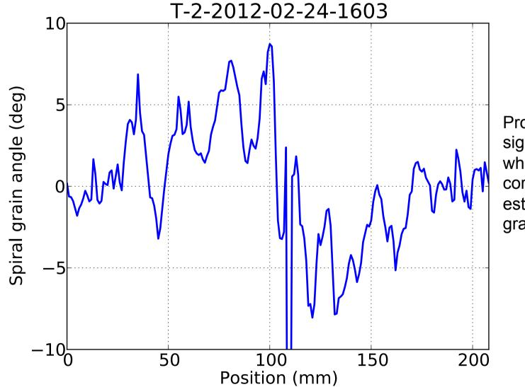
Processing the signal differences when rotating the core we can estimate spiral grain.
