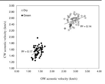
Fig. 7 Relationship between opposite wood (OW) and compression wood (CW) acoustic velocity for dry and green samples with the pooled data
