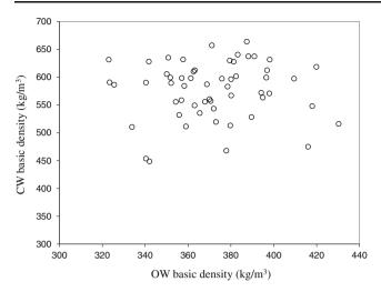
Fig. 5 Relationship between opposite wood (OW) and compression wood (CW) basic density with the pooled data
