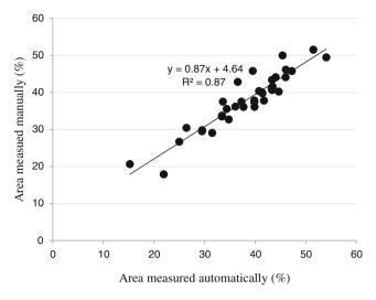
Fig. 4 Relationship between manually and automatically detected compression wood area in the disks. Manual detected values corresponded well with automatic detection
