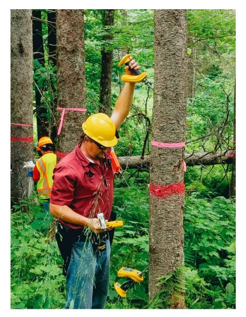
**Figure 2.** A portable time of flight (TOF) acoustic tool for measuring acoustic velocity (AV) in standing trees (photo credit: Xiping Wang).
