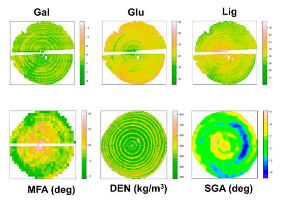
**Figure 16.** Examples of wood property maps produced by the DiscBot for galactan content (Gal), glucose content (Glu), lignin content (Lig), microfibril angle (MFA), density (DEN), and grain angle (SGA).
