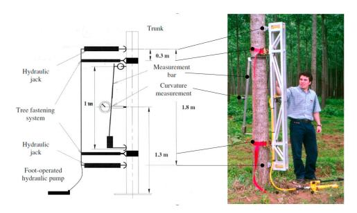
**Figure 6.** Characteristics of the Rigidimeter in its final version (from Pâques and Rozenberg, 2009) and setting up in an experimental trial of *Populus* in Chile.
