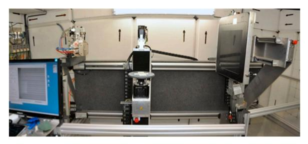
Figure 17. A micro-computed tomography (μCT) system in use at Ghent University [285].
