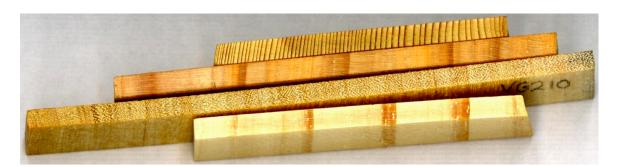
Figure 7. Samples prepared for SilviScan analysis.
