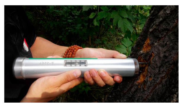
Figure 3. The Pilodyn wood tester (photo credit: Shan Gao).
