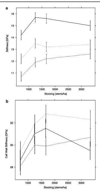
**Fig. 1** Outerwood stiffness (**a**) and cell wall stiffness (**b**) for *E. cloeziana* (solid line), *E. dunnii* (*dashed line*) and *E. pilularis* (*dotted line*) across four stocking levels. When considering basic density and wood stiffness together to calculate cell wall stiffness, the differences between species are reduced. In addition, the relative rankings change
