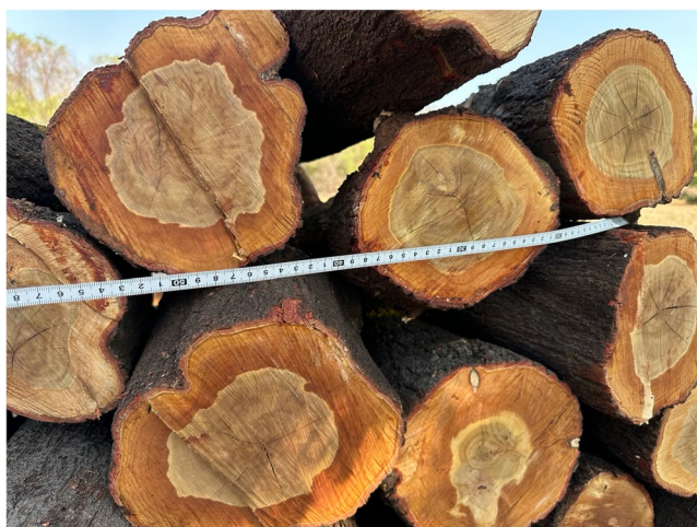
Fig. 1 An example of heartwood development in 13-year-old Indian sandalwood trees established in Northern Australia (courtesy: Dan Firth, Apical Forest management)
