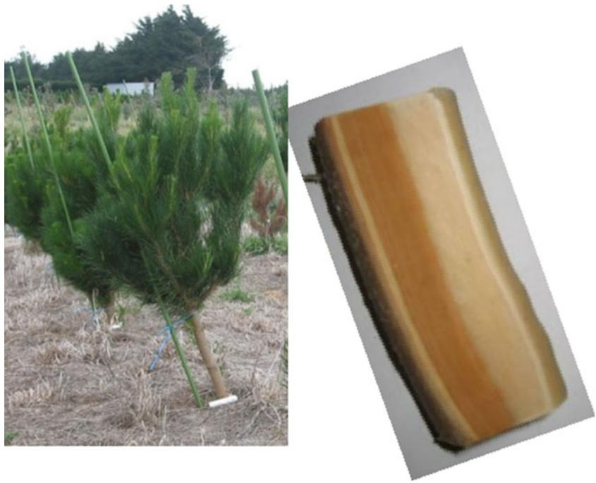
separately for “opposite” (upper side) and “compression” (lower side of sample) wood for green and dry acoustic velocity ( $\text{km s}^{-1}$ ), longitudinal shrinkage (%), volumetric shrinkage (%), and basic density ( $\text{kg m}^{-3}$ ).
